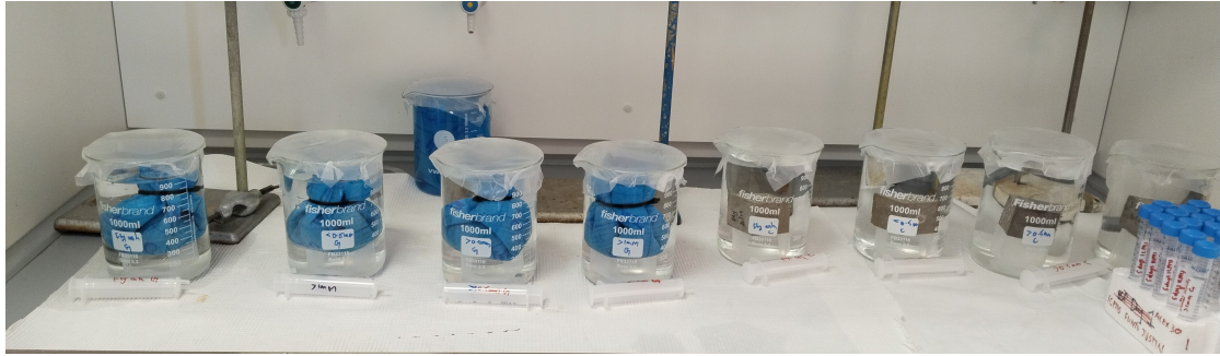
Figure 2.3: Experimental setup for Batch leaching Test
