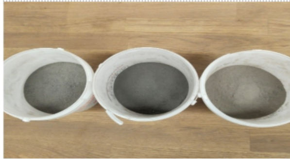
Figure 2.1: Ball milled MIBA samples from left >1\text{mm} , > 0.5\text{mm} and < 0.5\text{mm}
