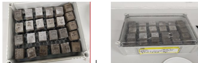
Figure 2.2: Curing of cubes without Submerging them in water
