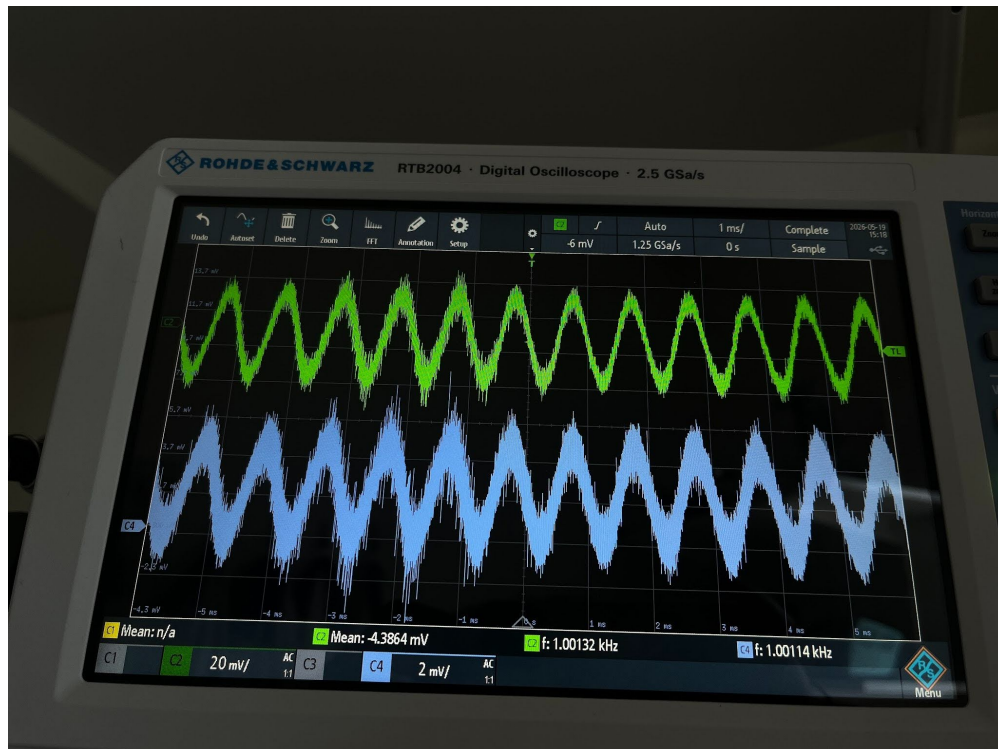
Figure 5.3: Guitar input signal at J2 (Ch2) and op-amp non-inverting input pin 3 (Ch4) at 1 kHz. Frequencies match (1.00 kHz), confirming AC coupling through C1 and signal transmission through the input network.
