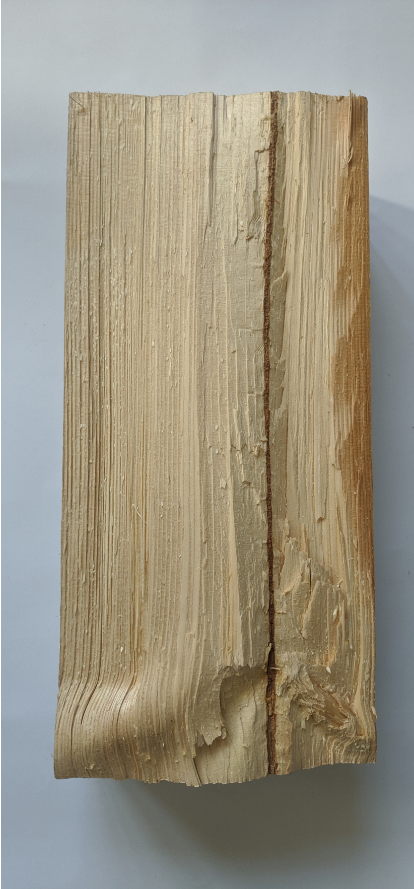
Pictures of two physical cleaving tests. The left from a piece of timber, 200x200mm, and the right a small 22x35mm stick.
