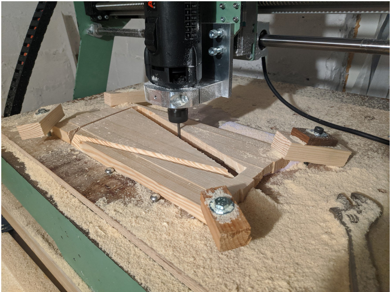
A typical setup for fabricating the pieces. There are four clamps and a foam shim visible in the back.
