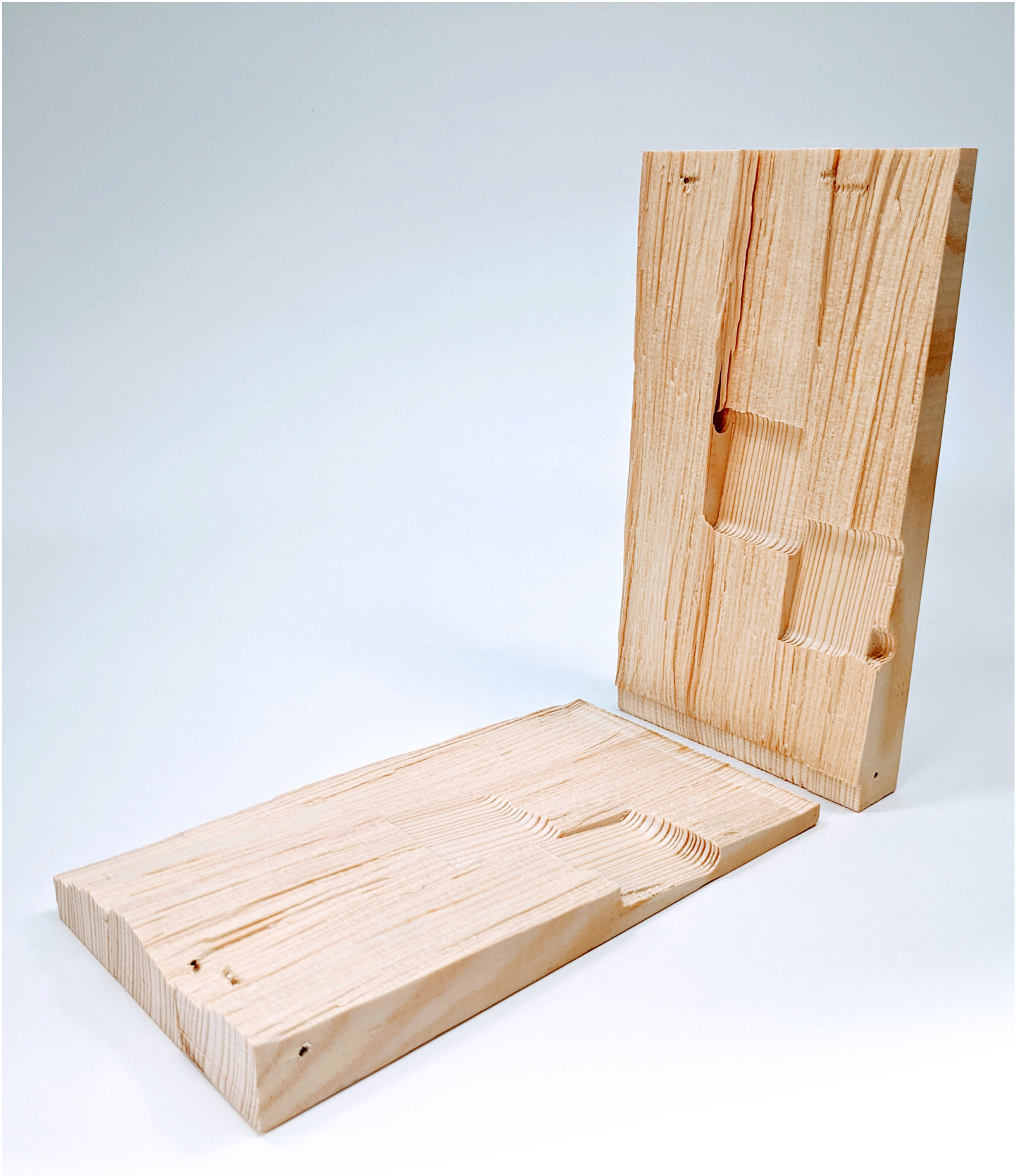
Only successful combination scale test that moved the cleave using pockets
