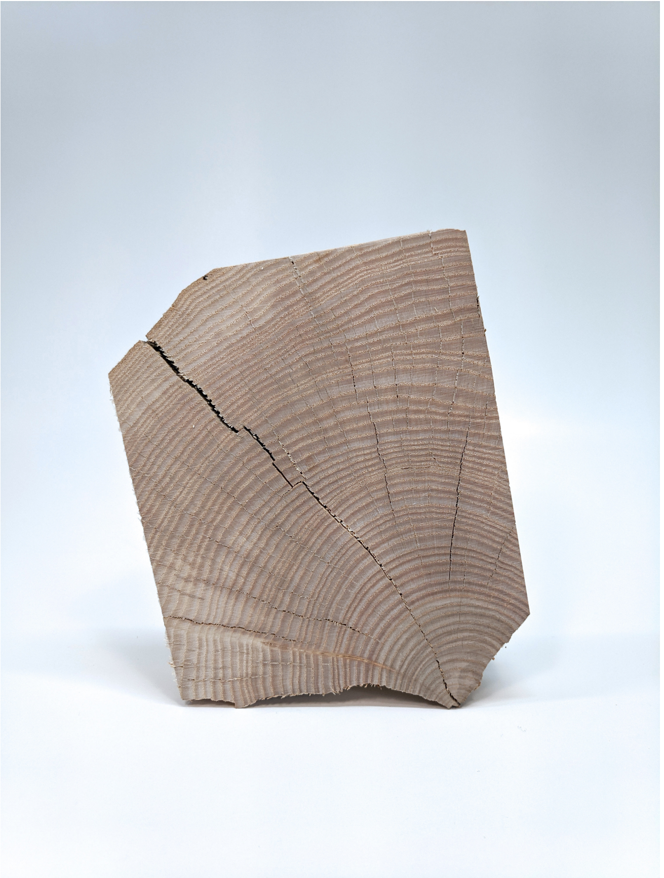
A slice of walnut timber, showing a crack propagate through the piece. The shape and direction is based on the grain structure formed when the tree grew, but also allows for a non linear split due to irregularities of a natural material.
