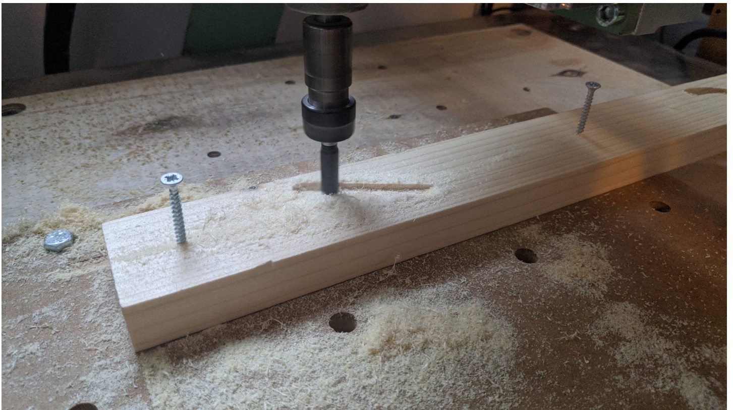
Above: CNC router that is used for physical testing Bellow: The actual routing of a pocket for a
