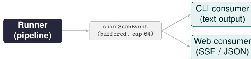
Figure 4.1: The typed event channel decouples pipeline execution from output. The Runner emits ScanEvent values into a buffered channel. Both the CLI and the Web-UI consume the same events independently.
