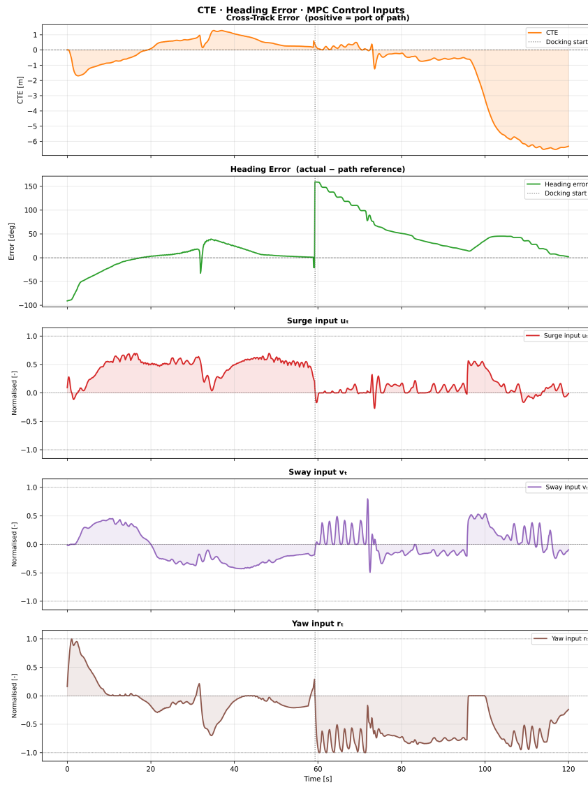
Figure 4.27: Plots of CTE, heading error and the corresponding control inputs.
