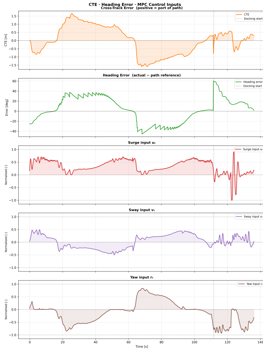
Figure 4.23: Plots of CTE, heading error and the corresponding control inputs.
