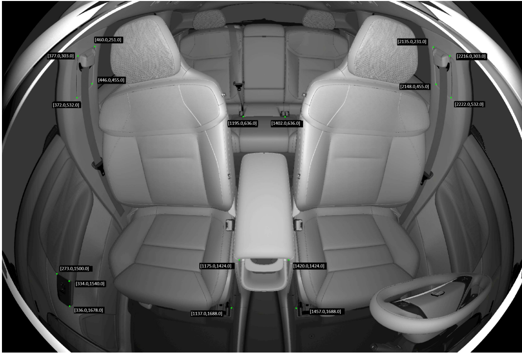
Figure 3.14: The nominal synthetic image with the landmarks highlighted in green with their location in the image.
