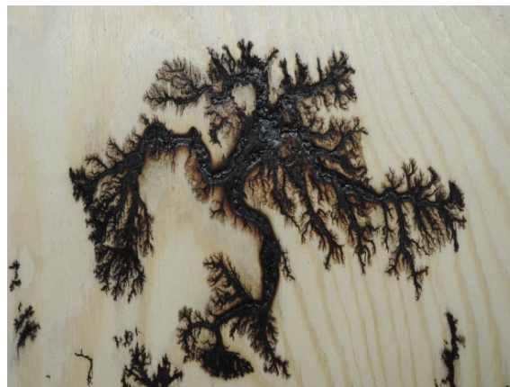
Figure 2.8: Visualization of tracking in the form of a Lichtenberg figure on a panel of wood. Image credit: (Helebrant, n.d.)
