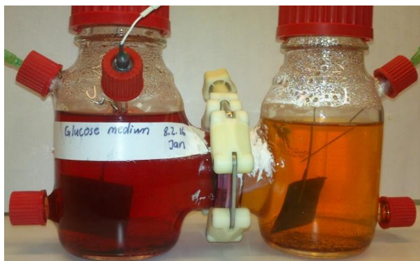
Figure 64: Reactor with glucose medium and neutral red mediator 3 days after inoculation.
