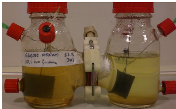
Figure 65: Picture of reactor with glucose media and neutral red mediator 54 days after inoculation.
