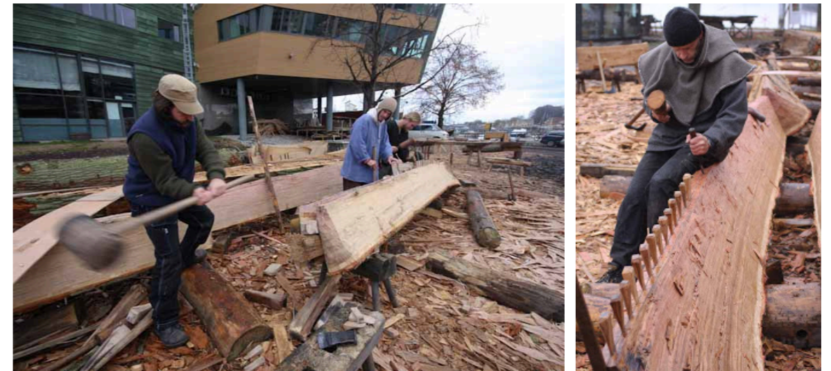
Diagonal oak cleaving, with control wedges along the length of the tree to ensure a continuous split
