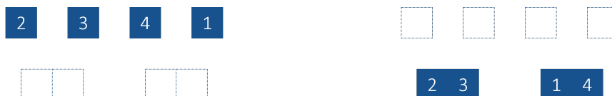
Figure 2.1: In this image a list with the elements 2,3,4, and 1 has been divided into sublists only containing one element. Thereafter the first two sublists are compared with the conclusion that 2 < 3 , merging them to the sublist \{2, 3\} . Similarly, \{4\} and \{1\} are merged to the sublist \{1, 4\} .
