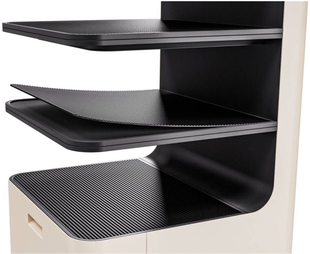
Figure 25 - Detachable silicon cover.
