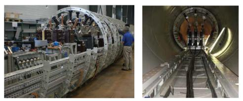
(a) A pre-assembly of the complete subsea (b) Beginning to install components switchgear system for testing. inside the cylindrical tank.
