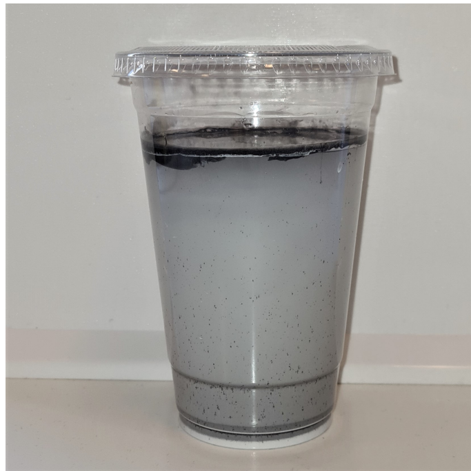
Figure 4.2: Storage stability sample of wood protection containing polyurethane 1 after 1 month of storage.
