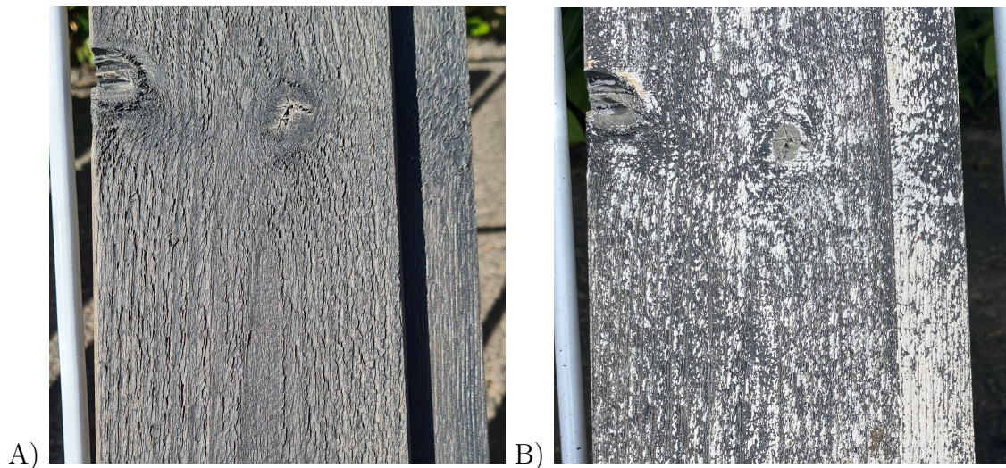
Figure 4.11: Fine sawn wood board coated with a with a sample of the reference: wood protection containing clay 1 and pigmented surface protection used in the natural weathering test. A) is before the test and B) is after 1 month of weather exposure.
