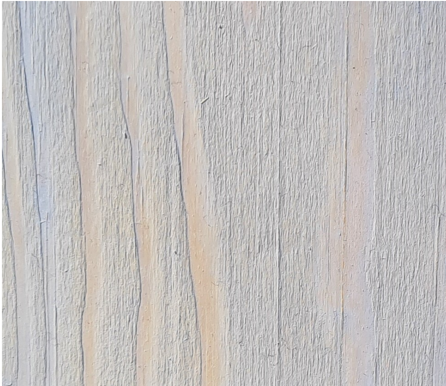
Figure 4.8: Planed wood board coated with wood protection containing clay 3 and unpigmented surface protection with an uneven distribution of pigment or wood protection.
