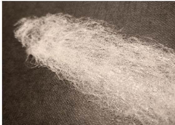
Figure 1: An example of a cellulose-based nonwoven material produced with solution blowing.
