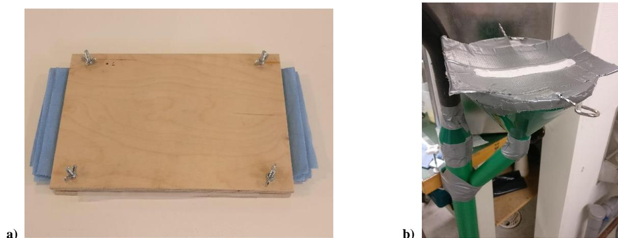
Figure A.1: a) One of the flower presses used during the drying of some of the cellulosic nonwoven samples produced in the project. b) The funnel construction used for vacuum drying of the samples. A vacuum machine was used to draw the liquid out of the samples placed on top of a mesh on top of the funnel.
