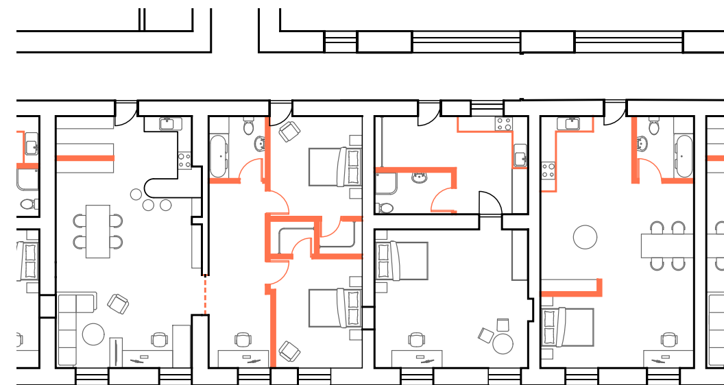
Figure 44: Social housing on the first floor, highlighting three types of apartment use: double apartment; single occupancy with wall division; single occupancy studio apartment
