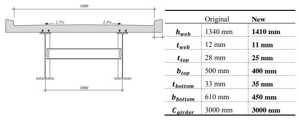
Figure 9.4 New bridge cross-section with dimensions
