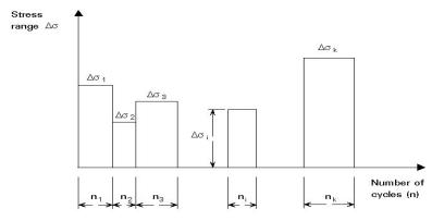
Figure 5.8 Stress histogram or stress range distribution used to simplify the loading amplitude history of a detail
