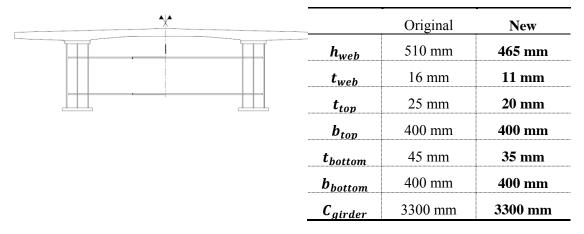
Figure 10.3 New bridge cross-section with dimensions (kept constant for support and span)
