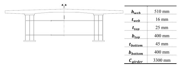
Figure 10.2 Bridge cross-section with dimensions
