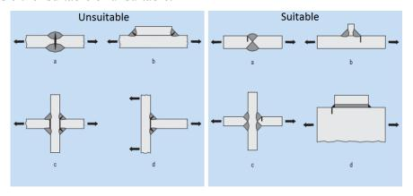
Figure 6.3 Suitability of application of HiFIT for different welded details
