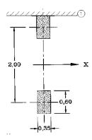
Figure 7.2 Tire size for LM2 (EN 1991-2, Figure 4.2b)
