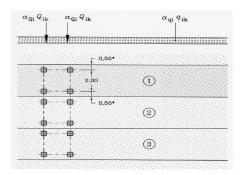
Figure 7.1 Traffic load distribution-transverse section (EN 1991-2, Figure 4.2a)
