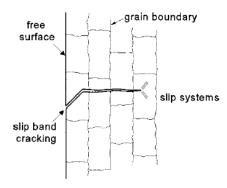
Figure 5.2 Path of a micro-crack through the cross section
