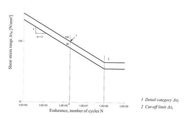
Figure 5.7 S-N curves for details loaded in shear
