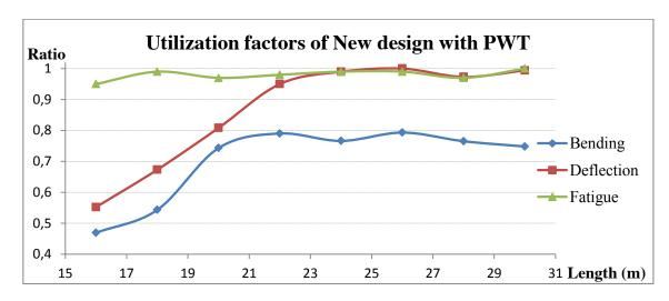
Figure 8.8 Utilization factors of New design with PWT
