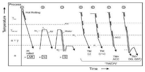
Figure 2.3 Temperature variation during the different possible heat treatment processes of High Strength Steel
