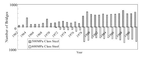
Figure 2.1 Number of bridges designed with High Strength Steel constructed in Japan over time
