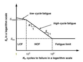
Figure 5.5 General S-N curve of a steel detail
