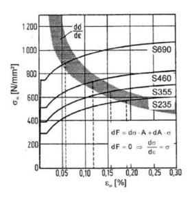
Figure 2.7 Stress-strain curves for different steel grades
