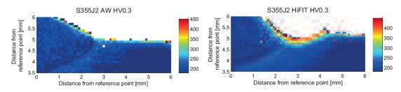
Figure 6.4 Strain hardening of the weld metal due to HiFIT
