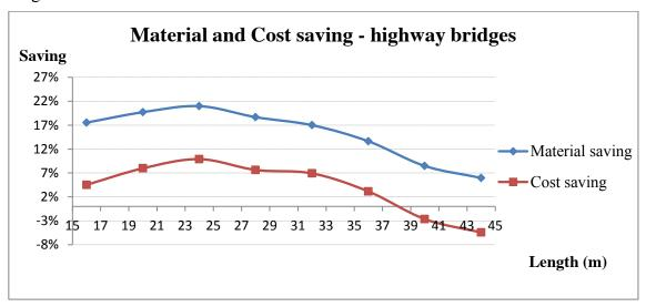
Figure 9.5 Material and cost saving achieved with the new design
