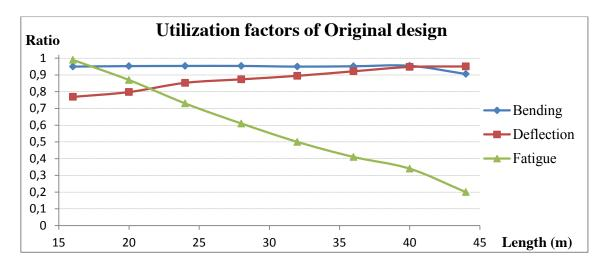
Figure 9.6 Utilization factors of Original design
