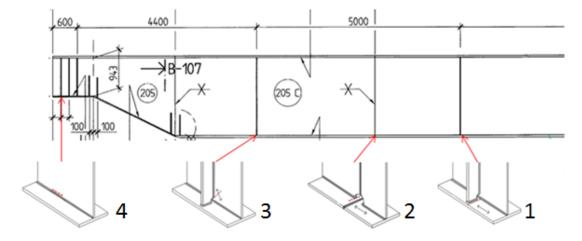
Figure 8.3 Detail view of the critical details for fatigue resistance
