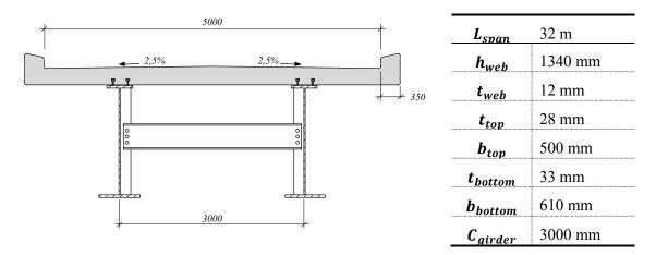
Figure 9.2 Bridge cross-section with dimensions
