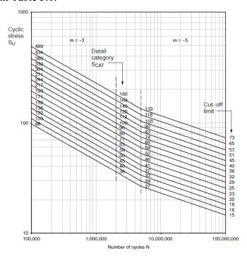
Figure 5.6 S-N curves for details loaded with normal stresses
