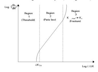
Figure 5.4 Typical fracture mechanics fatigue crack propagation behaviour
