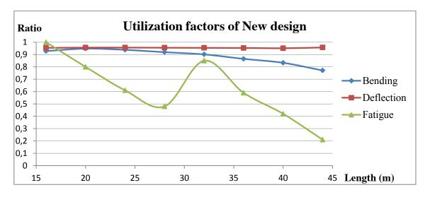
Figure 9.7 Utilization factors of New design with PWT
