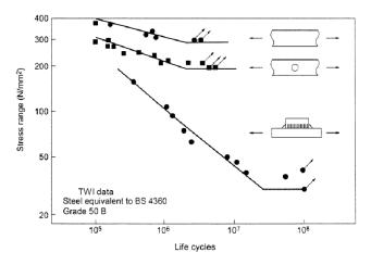
Figure 5.9 Fatigue life of plain specimens, compared to notched or welded
