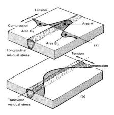
Figure 5.10 Residual stresses after welding both in longitudinal and transverse direction
