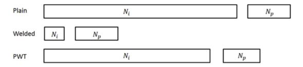
Figure 6.1 The benefit of PWT in restoring the crack initiation life of a welded specimen
