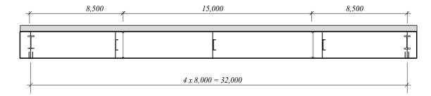
Figure 9.1 Longitudinal view of the highway bridge over E4 in Skulnäs, Sweden
