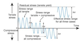
Figure 5.11 Effect of residual stresses on the position of the stress range
