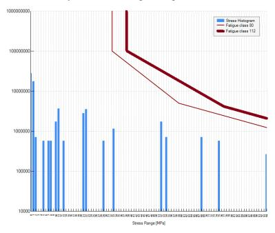
Figure 8.5 New position of the S-N curve after PWT
