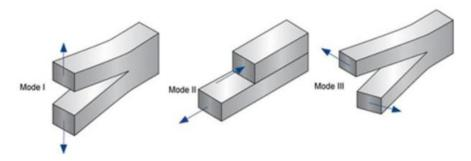
Figure 2.6 Possible modes of fracture propagation for metals
