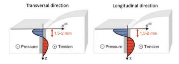
Figure 6.5 Depth distribution of stresses due to HiFIT both in transversal and longitudinal direction respectively
