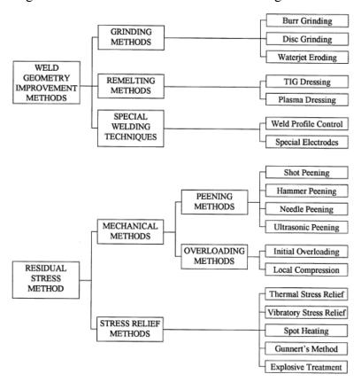
Figure 6.2 Classification of methods of post weld treatment
