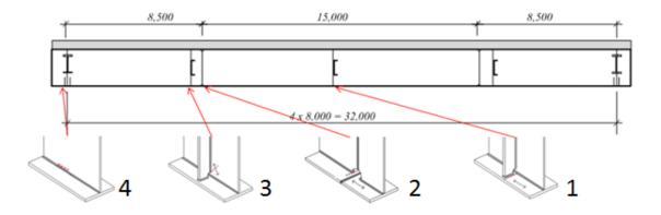
Figure 9.3 Detail view of the critical details for fatigue resistance
