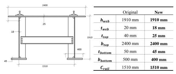
Figure 8.4 New bridge cross-section with dimensions
