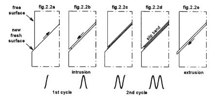
Figure 5.1 Shear stresses in the metal lead to the propagation of micro-cracks and the formation of a bond slip
