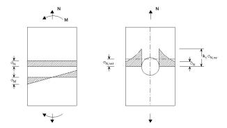
Figure 5.3 Plan view of nominal stress and geometric stress concentration of both a plain specimen and a plate with a hole
