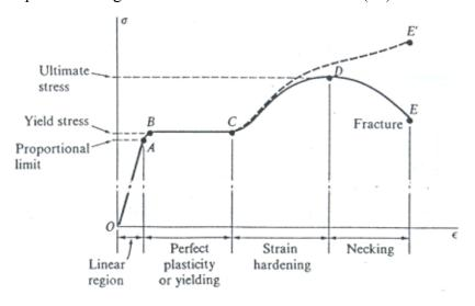
Figure 2.5 General stress-strain curve for steel
