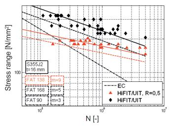
Figure 6.6 Comparison of fatigue strength between as-welded butt joints and HiFIT treated butt joints
