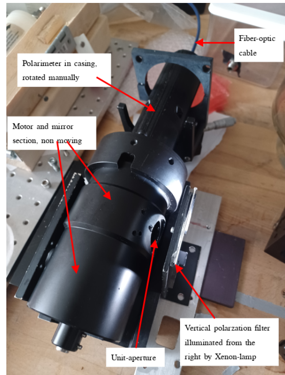
(b) Photo of the setup. The white frame contains the polarization filter.
