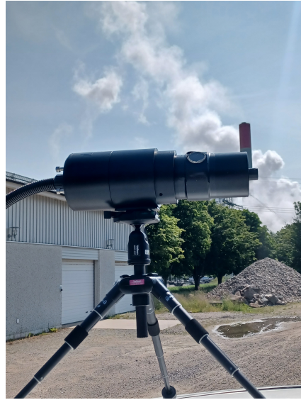
(b) Image of pulp mill and instrument direction. Note that the instrument only catches light falling parallel to the aperture direction so the chimney should not interfere with the measurement. The instrument was horizontal so the tilt is due to the camera.
