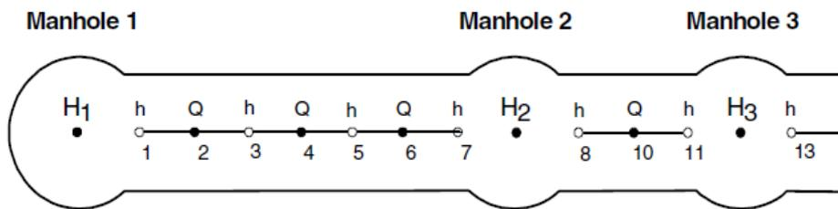
Figure 3-2. Computational grid in the pipe network, consisting of stacked points of  $h$  (water level in pipe) and  $Q$  (flow) (DHI, 2004).
