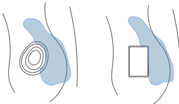
Figure 7-2. Schematic figure on surface water spread on DEM with different accuracy. For same conditions, the model to the left would be interpreted as flooded building whilst the model to the right would not.
