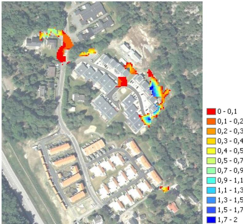
Figure 5-12. First 2D simulation results showing maximum flood depth in meters; a result that did not correspond with the real rain event. Scale is showing flood depth in meters.
