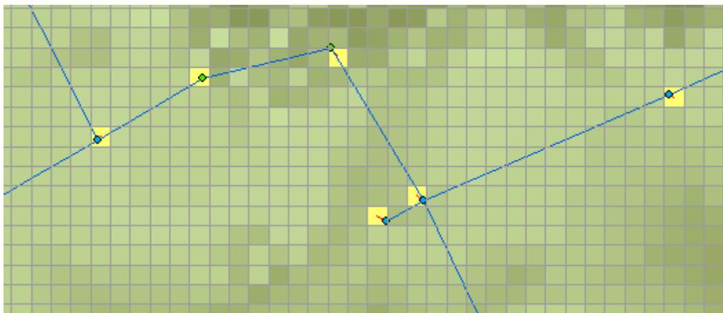
Figure 3-7. The network models manholes coupled to the grid squares in the digital elevation model.
