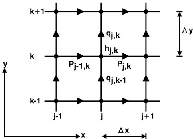
Figure 3-4. Difference grid showing the principle of the alternating technique for solving continuity and momentum conservation equations.  $p$  and  $q$  is the flux in the different directions, and  $h$  is the water level (Mike by DHI, 2011).
