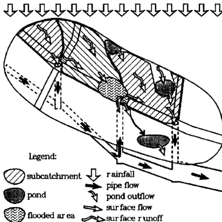
Figure 3-1. Conceptual figure over water flow paths during a rain event in an urban area. Water flows on both the surface and in the pipe network which has insufficient capacity which leads to flooding (Djordjevic et al 1999).
