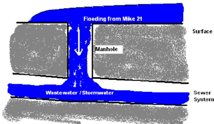
Figure 3-5. Overland flow reaches an open manhole which leads to an interaction where water is transported from the 2D model to the 1D model (DHI, 2007).
