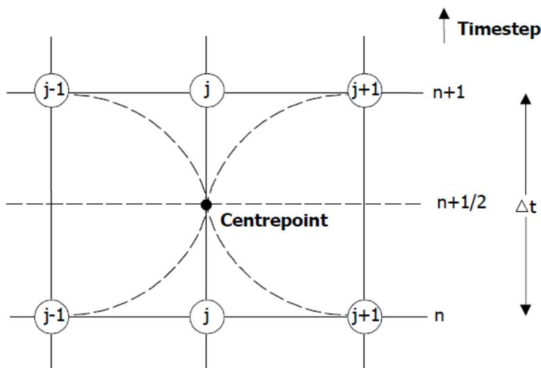
Figure 3-3. The principle of the six point Abbott scheme used for the finite differences approximation of the flow equations in the 1D model (DHI 2004).
