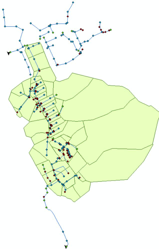
*Figure 5-7. The network model for the case area during the model building process. In the figure one can see closed manholes (blue), gully pots (red) and trench intakes (green). Yellow fields are catchments used in the time-area method and the black triangles are the outlets where the model ends.*
