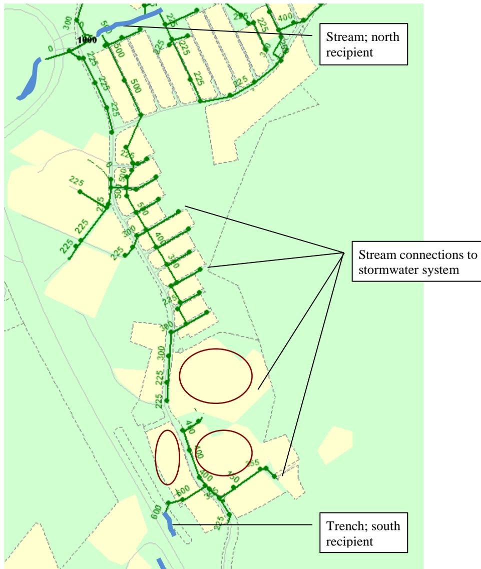
*Figure 5-2. The storm water system for the studied area of Kopparkärret. In the area there are three joint properties, marked with ellipses, whose systems are not included in Gothenburg Waters databases. Note that the system is divided into a north and south part (Göteborg Vatten, 2012b).*
