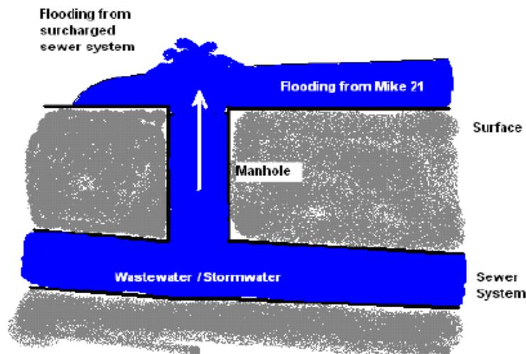
Figure 3-6. The capacity in the storm water network is reached which leads to an interaction where water is transported from the 1D model to the 2D model (DHI, 2007).
