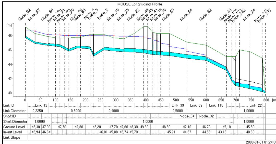
Figure 5-11. First model results from 1D network simulation, north part of stormwater system. Pressure line exceeds ground level which was according to the real rain event.
