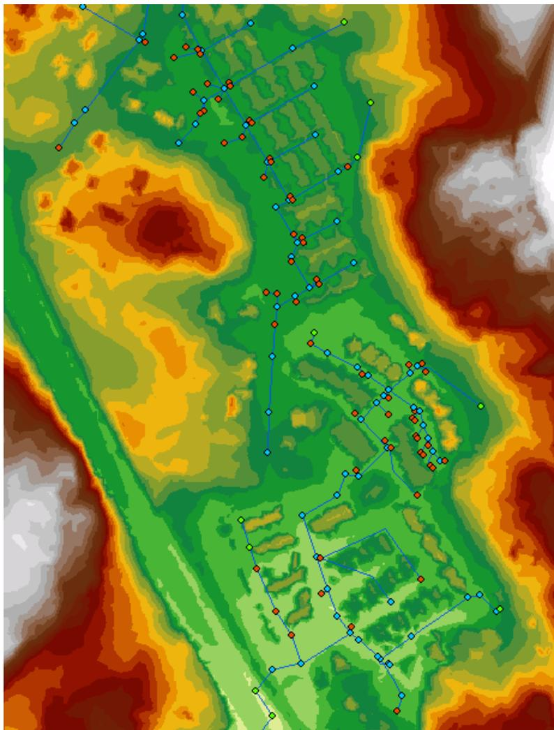
*Figure 5-9. The 1D network model coupled with the 2D elevation model.*
