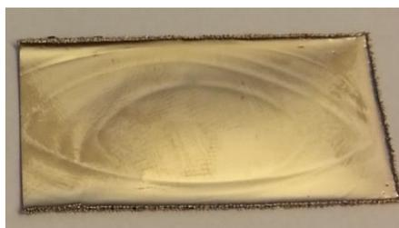
**Figure 5: Waviness of the sample produced at 20 A/dm<sup>2</sup> and 35 °C.**
