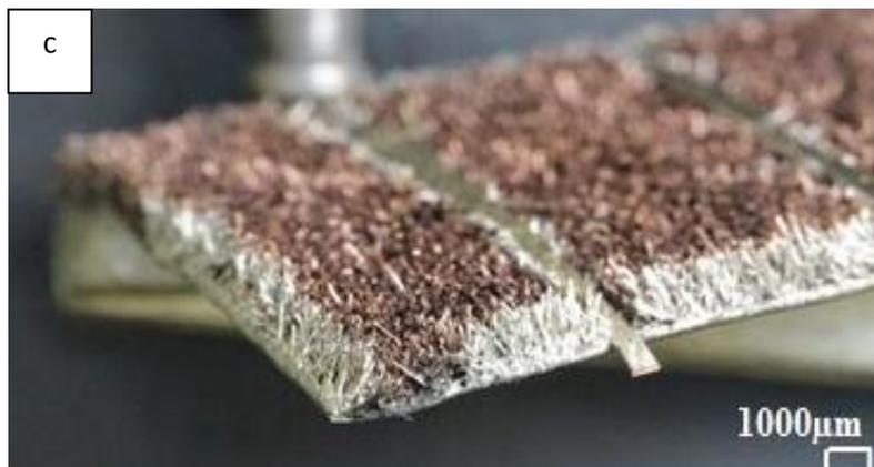
**Figure 28: Electrodeposition of Nickel on polymer fibers a) Cross section image showing fibers after Gold sputtering, b) Cross section image showing the electrodeposited Nickel coating on fibers, and c) Image showing the electrodeposited Nickel coating on fibers at the sample edge and close to the attached copper wires.**
