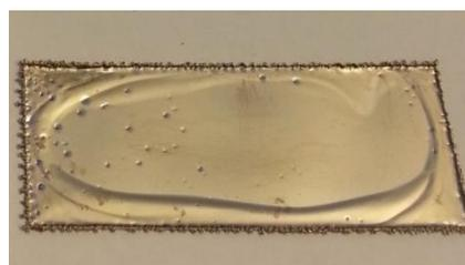
**Figure 6: Pitting observed in the sample produced at 20 A/dm<sup>2</sup> and 45 °C.**
