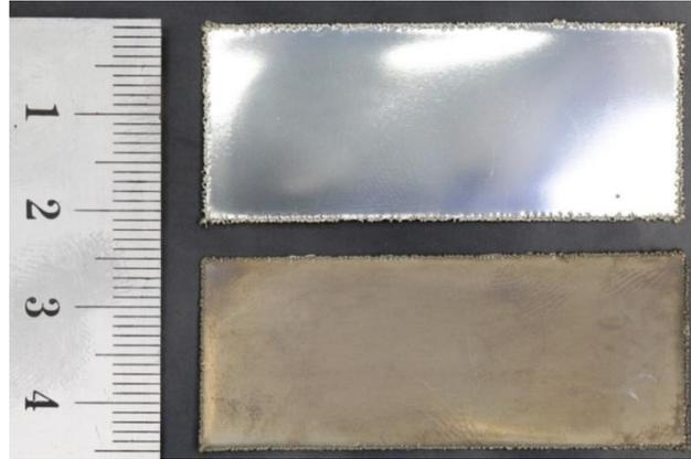
**Figure 7: Comparison of the appearance of the samples produced under the same plating condition with Electrolyte I (Top) and Electrolyte II (Bottom).**
