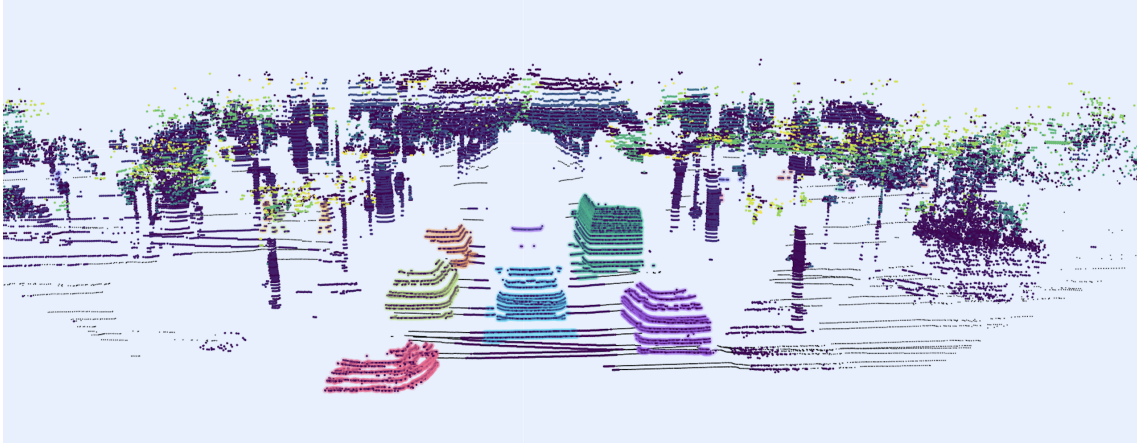
Figure 5.2: Visualization of Point Cloud with Ground Truth Annotations. Colored points represent different clusters. Semi-transparent overlays highlight ground truth object labels derived from bounding boxes.
