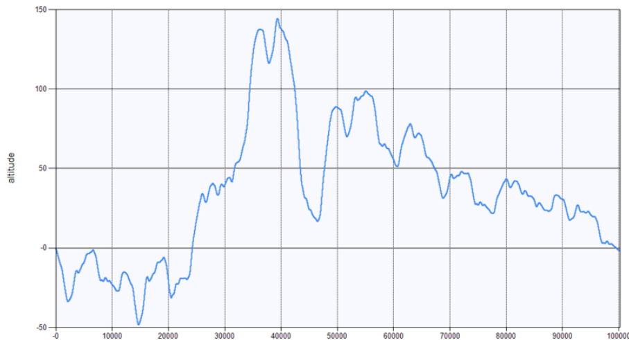
Figure 7.1: Reconstructed road altitude profile derived from VECTO gradient data.
