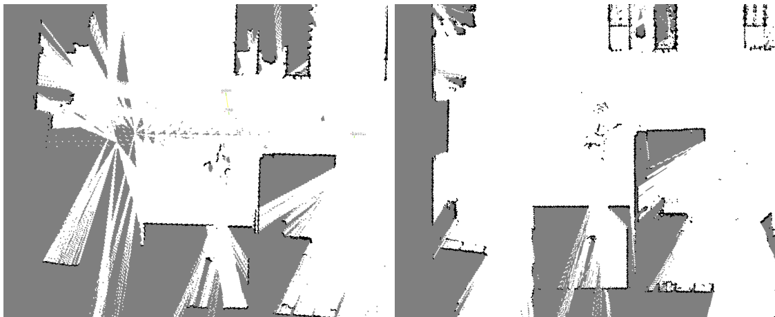
Figure 4.10: Map of an indoor industrial environment generated with SLAM Toolbox, utilising the dynamic filter with POG classification on the left and POI classification on the right.
