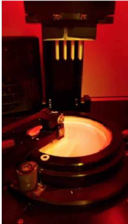
Figure 7: A completed printing process where the bending bars have been printed in a standing fashion.
