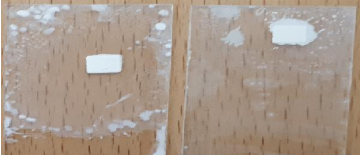
Figure 2: Two samples for investigating overcuring. Notice the imperfection around the right sample. It has been overcured.
