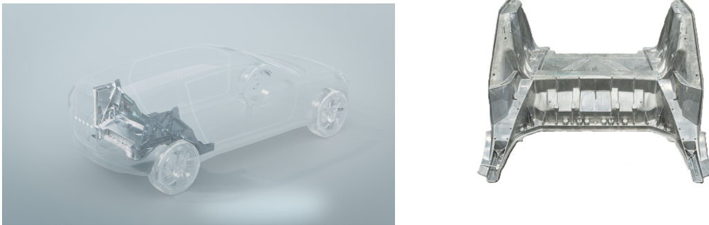
(a) Rear floor positioned in car, from [1]. (b) Mega-cast rear floor, adopted from [2].
