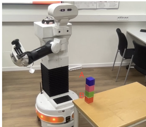
Figure B.14: Depiction of the trace cube stack task. The task was to teach the robot to trace the stack of cubes by first going to a grasp pose for cube ‘A’ and then trace the stack down to cube ‘B’ and up again.
