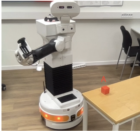
Figure 3.10: Depiction of the grasping task. The task was to teach the robot to get into a grasping pose for the red cube marked by a red ‘A’.
