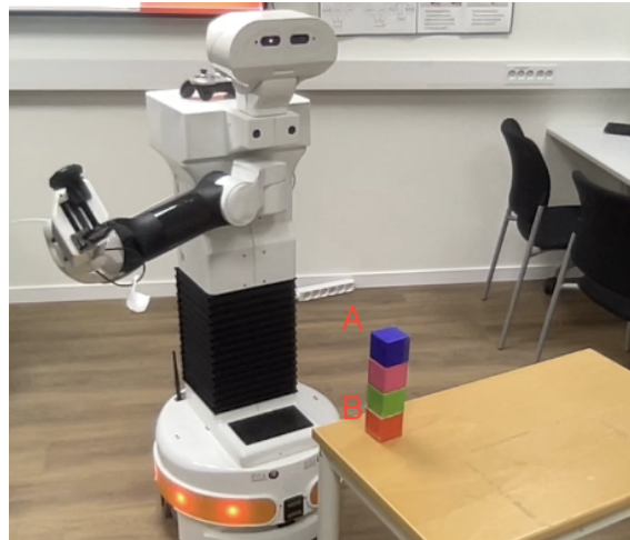
Figure 3.4: Depiction of the trace cube stack task. The task was to teach the robot to trace the stack of cubes by first going to a grasp pose for cube ‘A’ and then tracing the stack down to cube ‘B’ and up again.
