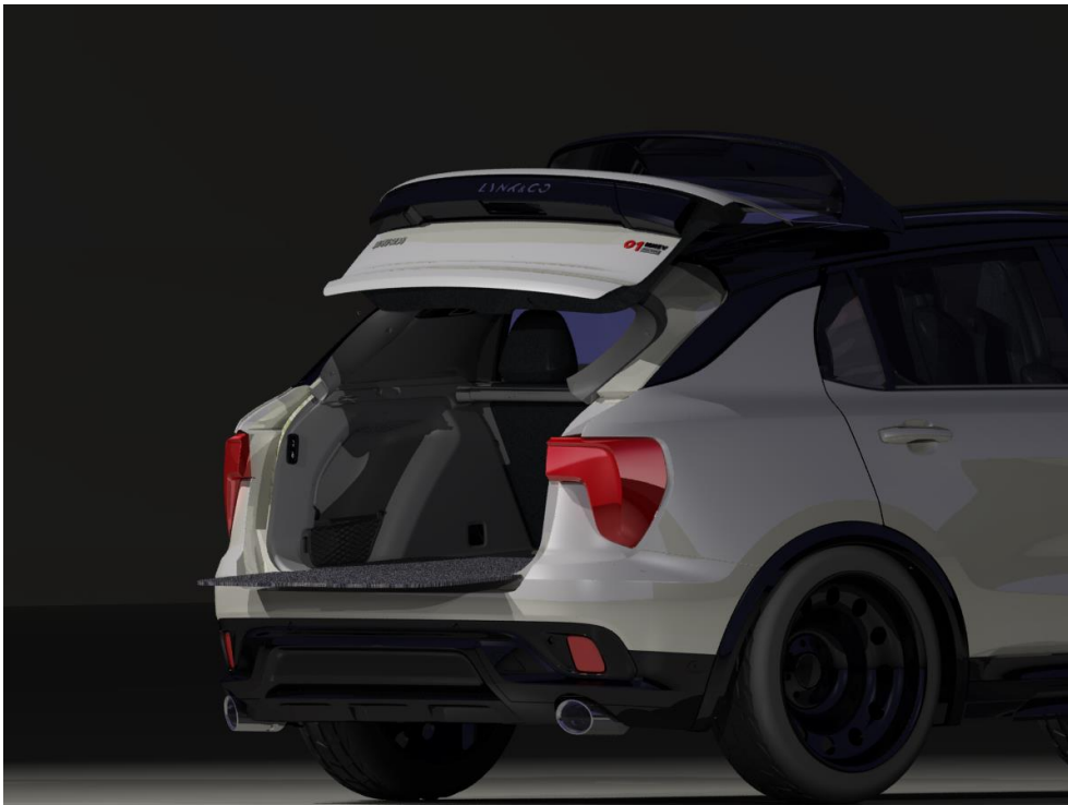
Figure 39 - Perspective view 2 of the new tailgate solution.
