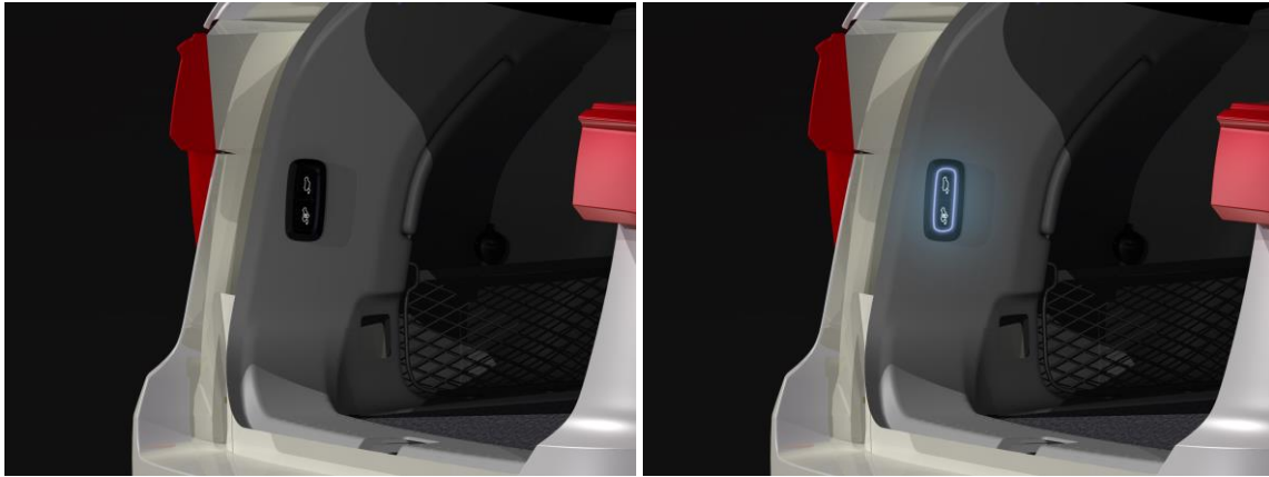
Figure 54 - Illuminated tailgate operation control, close-up view.
