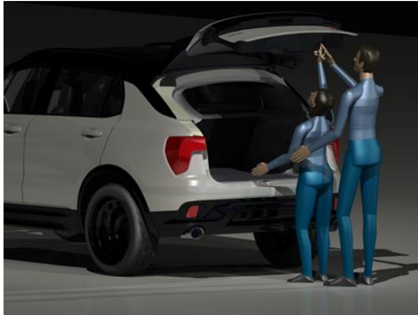
Figure 3 - Ergonomic simulation of three mannequins (Woman, German, 5-50-95 percentile) using the luggage space of a Lynk & Co 01.
