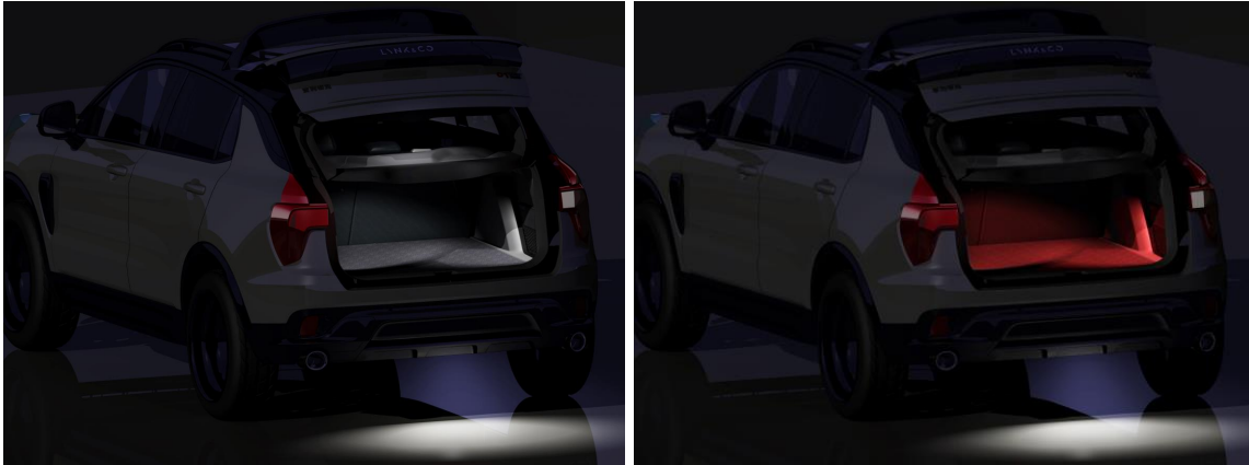
Figure 55 - Visual feedback by changing the light's characteristic (Tailgate closing).
