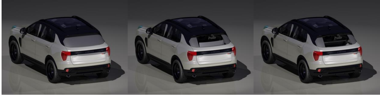
Figure 48 - The fold-down process of the power-operated tailgate window.
