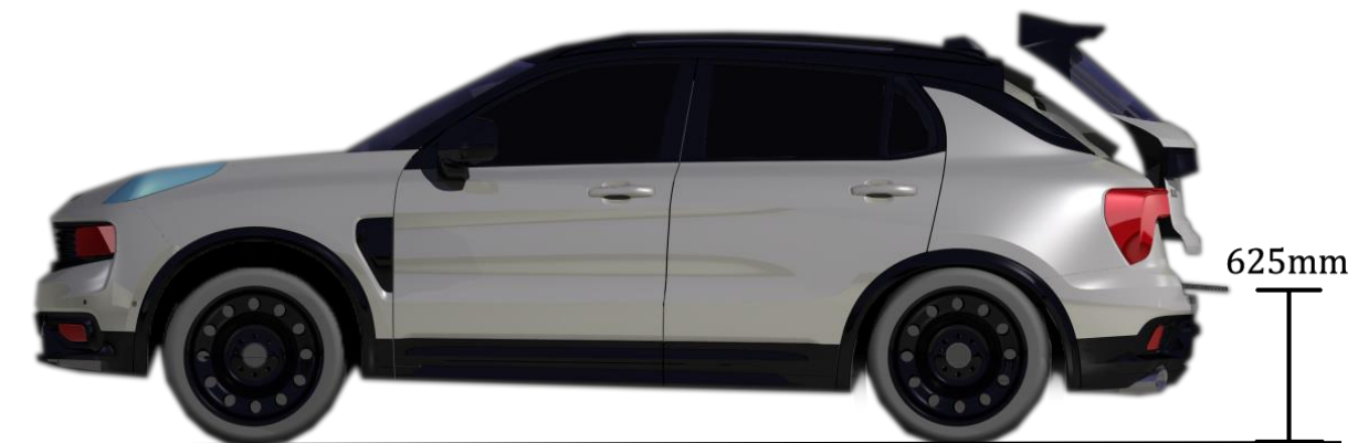
Figure 47 - Lift-in-height with deflated air suspension.
