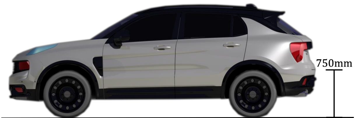
Figure 46 - Lift-in-height with inflated air suspension.
