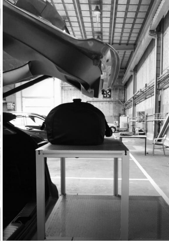
Figure 58 - Tailgate equipped with obstacle detection sensors, stopping at a safe distance to the object.
