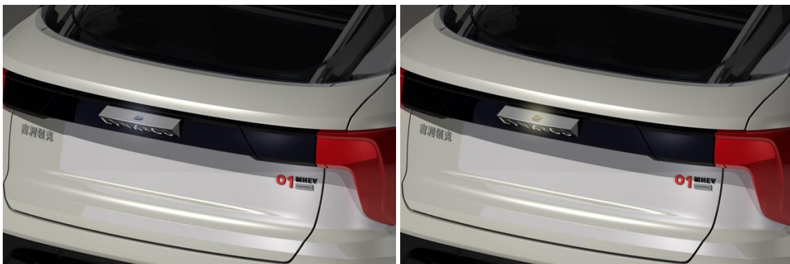
Figure 57 - Visual feedback by changing the light's characteristic (Tailgate opening).
