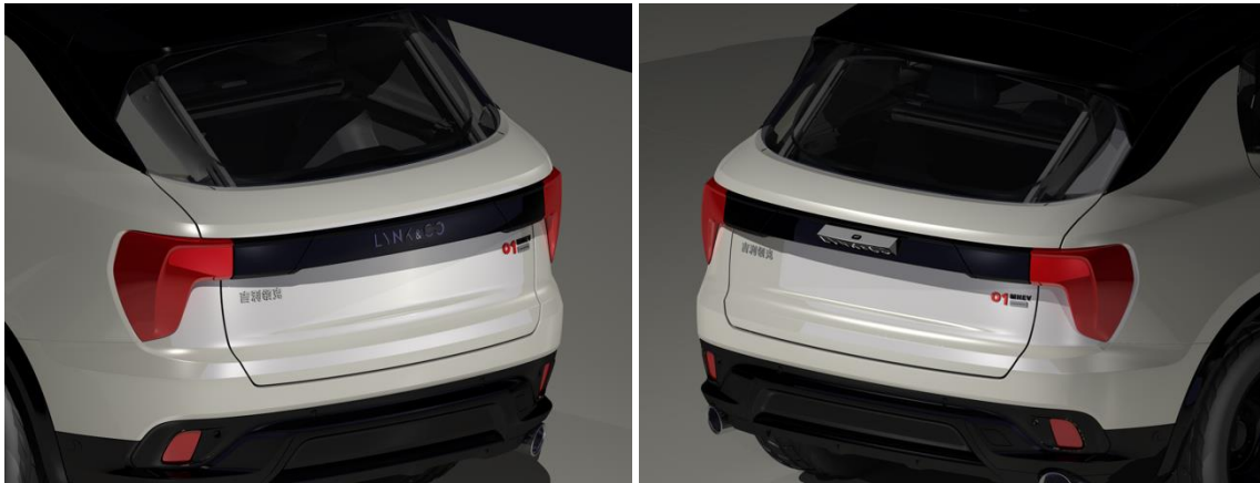
Figure 41 - (Left) illustrates the design when the opening button is hidden. (Right) illustrates an open hatch.
