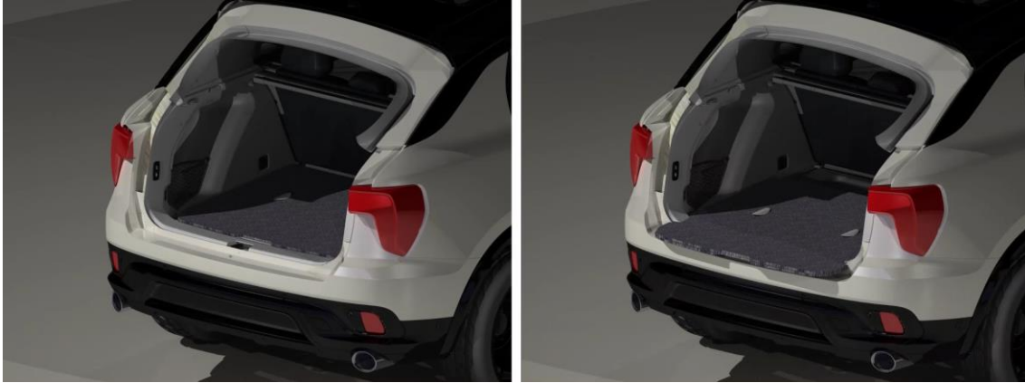
Figure 49 – Power-Operated floor positioned in its extreme translations.
