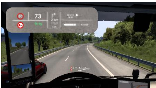
Figure 24. Highway mode base-HUD with constant elements and two temporary elements (road sign and adaptive cruise control). Reprinted with permission.
