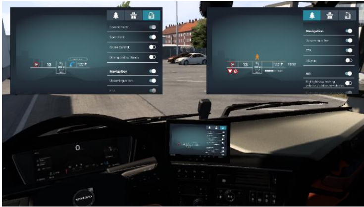
Figure 21. HUD setting on the secondary display. Two versions with different selections. Reprinted with permission.
