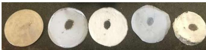
**Figure 4.6:** Disassembled cell components (SS disk, 3 separators and Mg foil from left to right) of a short-circuited cell cycled with E4 medium M4 concentration. Dendrites have pierced the separators.
