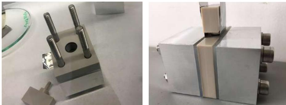
**Figure 3.3:** Conductivity cell assembled and disassembled. Electrolyte is only in contact with walls of plastic mid-section, cap and current collectors.
