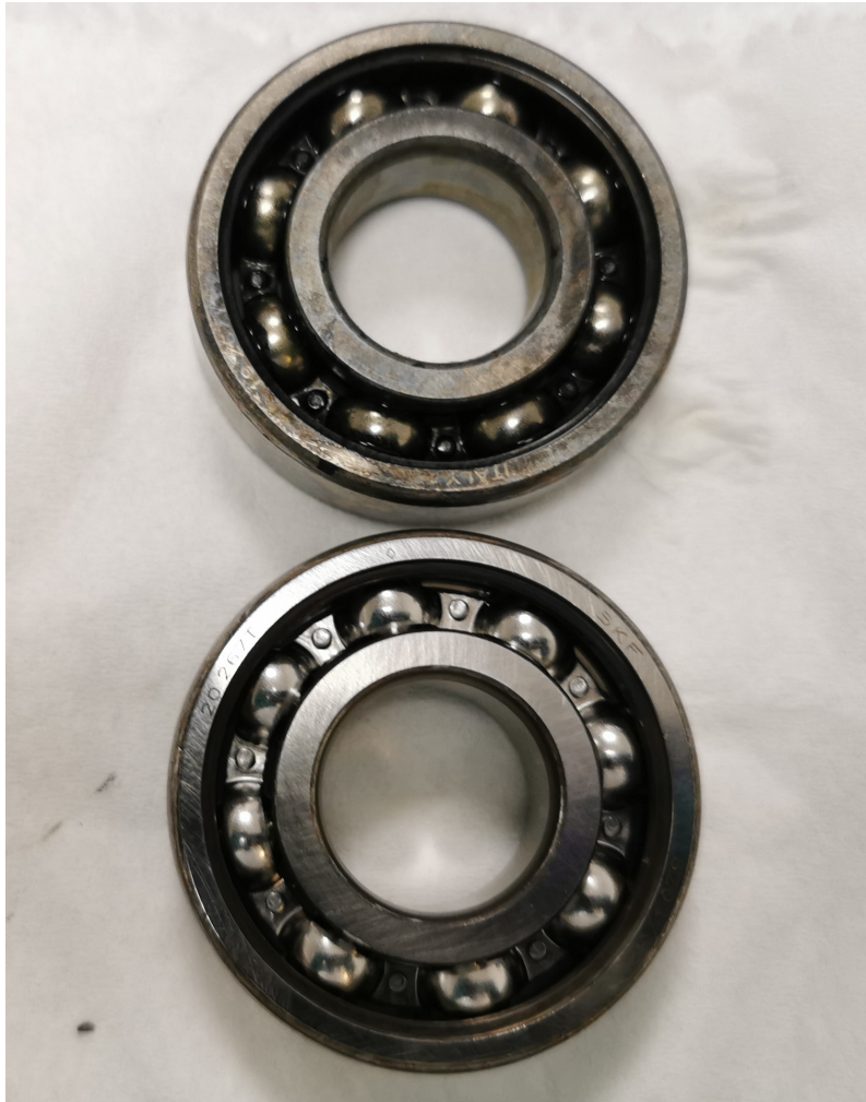
Figure A.2: Comparison between bearing fully submerged and charged for one hour at 80°C (upper) and an uncharged bearing (lower)
