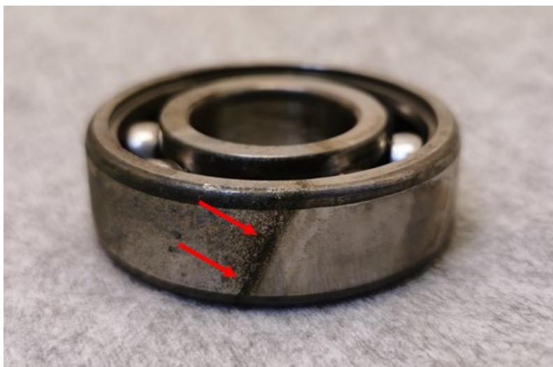
Figure A.1: Waterline corrosion seen on the bearing charged indicated while only being halfway submerged. The waterline is indicated by the arrows
