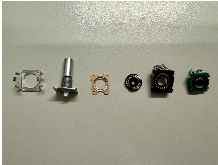
Figure 5.4: Rotary encoder internals.
