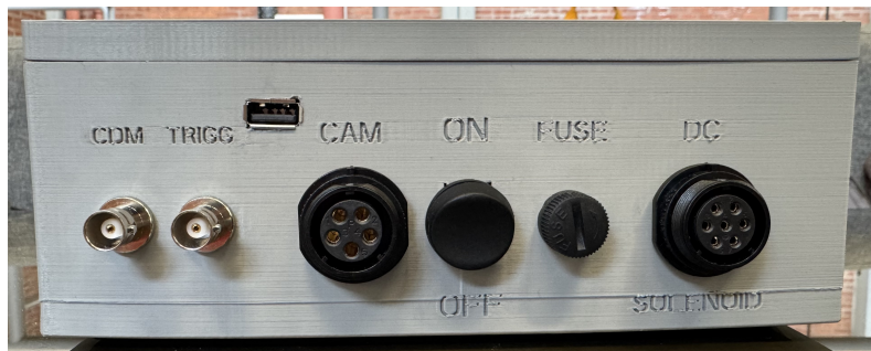
Figure 5.5: Rear of box with connectors.
