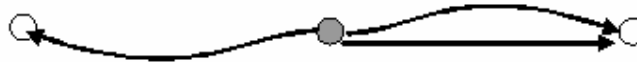
Figure 3: The dark one is the current node which points to un-removed node to its left and its right. It also points to the next immediate node.
