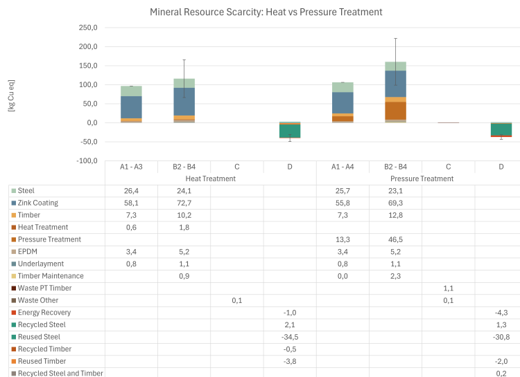
Figure 4.13. Results for mineral resource scarcity of heat-treated vs. pressure-treated timber for complete bridges, including TRP deck, timber railing, and superstructure.
