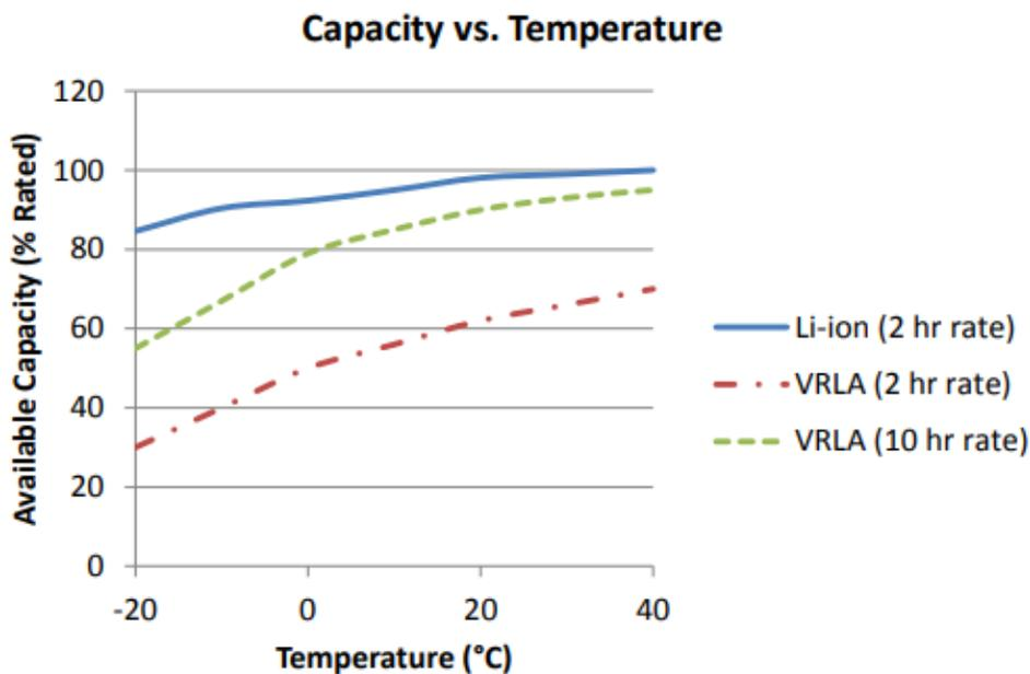
Figure 9 in cold climates the capacity loses capacity (Albright et al., 2012). Reprinted with permission
