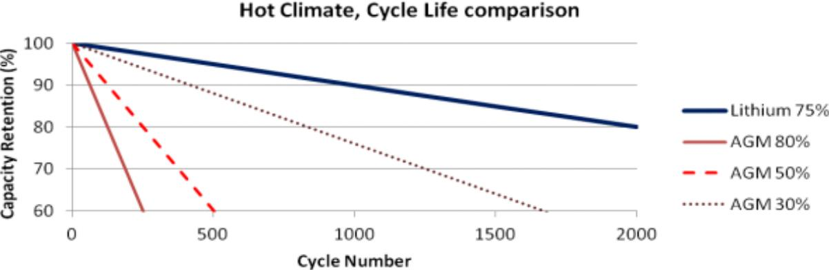
Figure 11 Cycles in hot climate around 33 Celsius (Albright et al., 2012) Reprinted with permission.
