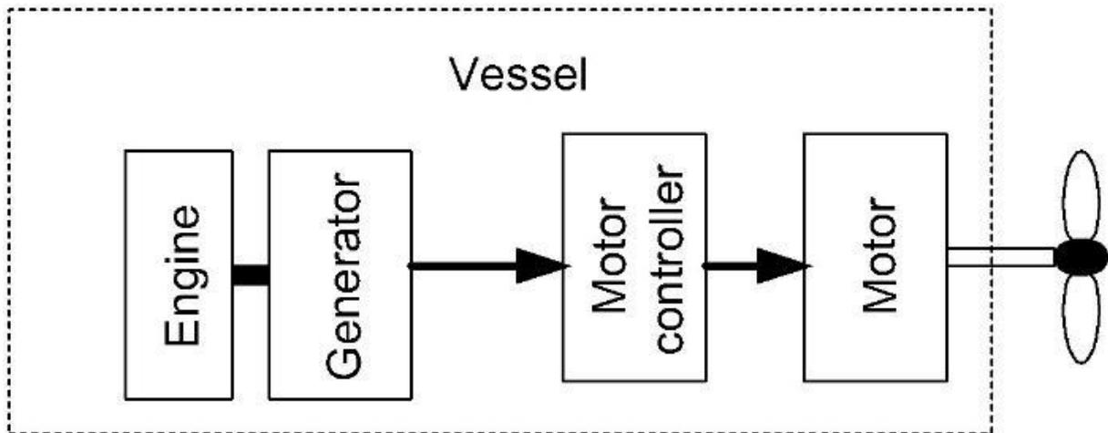
Figure 5 basic overview of a diesel/electric system and how it fits together. (Hybrid-Marine LTD, 2008) Reprinted with permission.
