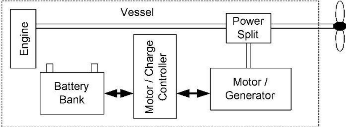
Figure 7 basic overview of a parallel hybrid. (Hybrid-Marine LTD, 2008) Reprinted with permission.
