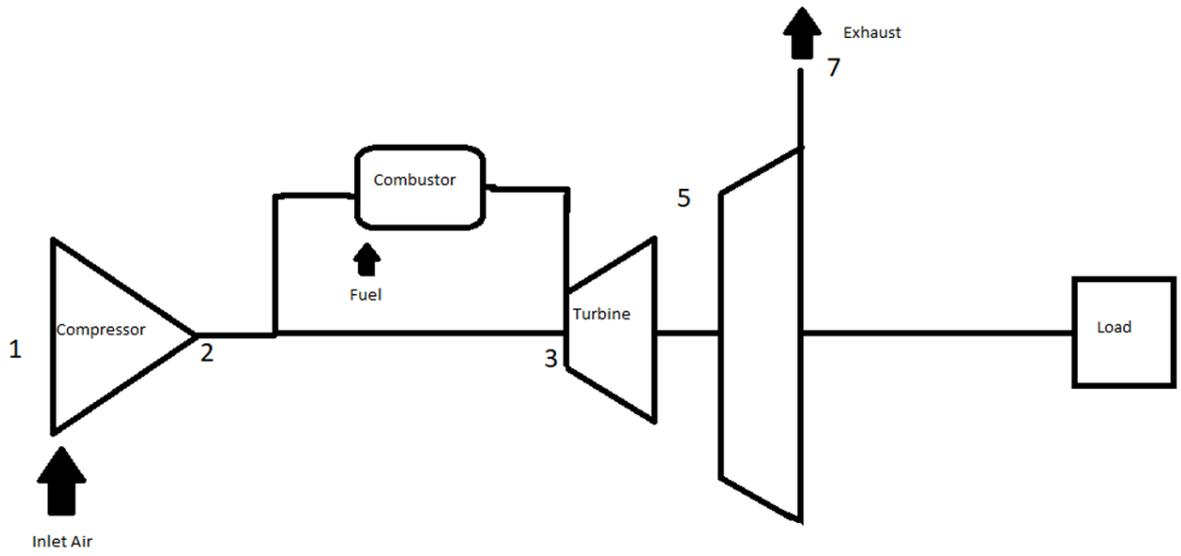
Figure 2 a simplified simple-cycle gas turbine principle. (Petrowiki, 2012. Authors own figure)
