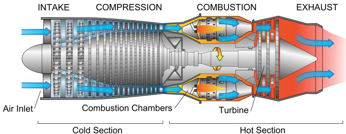
Figure 1 a cross section of a gas turbine to show how it works from the compression to the exhaust. (Wikipedia, reprinted with permission).
