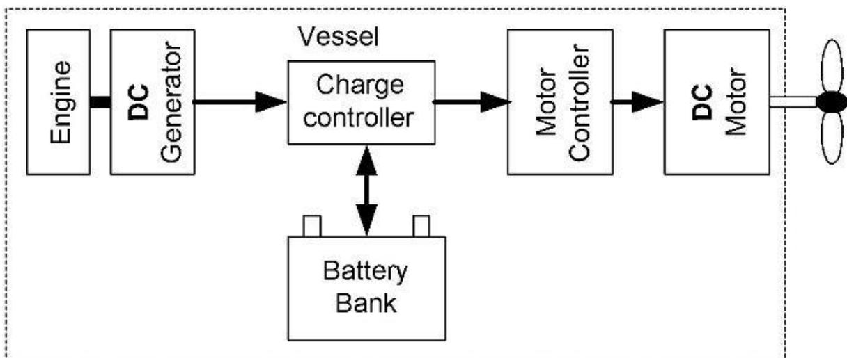
Figure 6 basic overview of a serial hybrid. (Hybrid-Marine LTD, 2008) Reprinted with permission.
