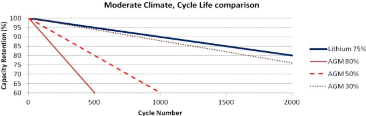
Figure 10 Cycles in moderate climate around 25 Celsius (Albright et al., 2012). Reprinted with permission.
