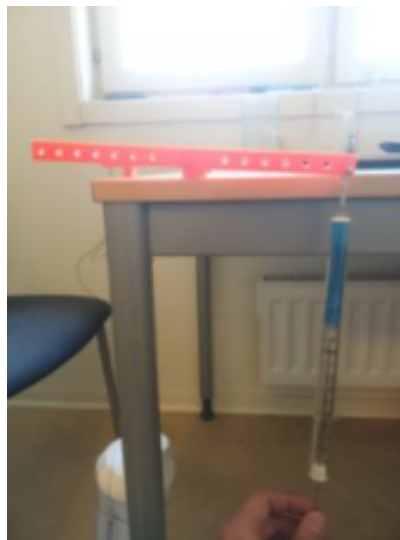
(b) Front view of the testing. Both the dynamometer and the load (water bottle) can be observed.
