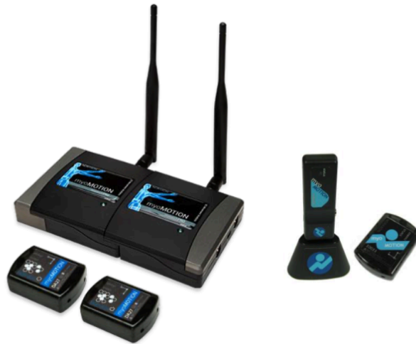
Figure 4.8: Noraxon myoMOTION inertial sensor system, including sensors and wireless modules. Note. Reproduced with permission from Noraxon USA Inc. (n.d.). Source: https://www.noraxon.com/download/myomotion-system-user-manual/?wpdmdl=18194
