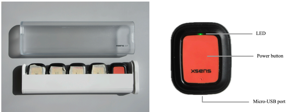
(a) Movella DOT sensor kit with included charger docking station and cover. (b) Parts of the Movella DOT sensor.
