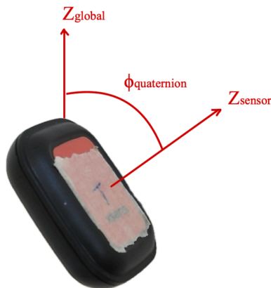
Figure 7.3: Illustration of quaternion based tilt, \phi_{quaternion} , defined as the angle between the sensor Z -axis and the global Z -axis.
