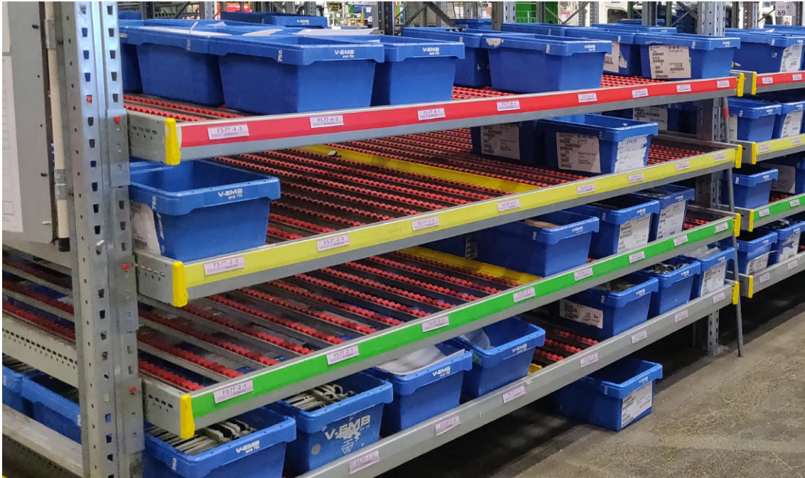
Figure 2.10: An image of four layers of gravity-fed conveyors, for the red racks, with boxes and stop edges. Where the edges have been colorized in order to visualize the ergonomic zones, which will be further described in Chapter 4.2.
