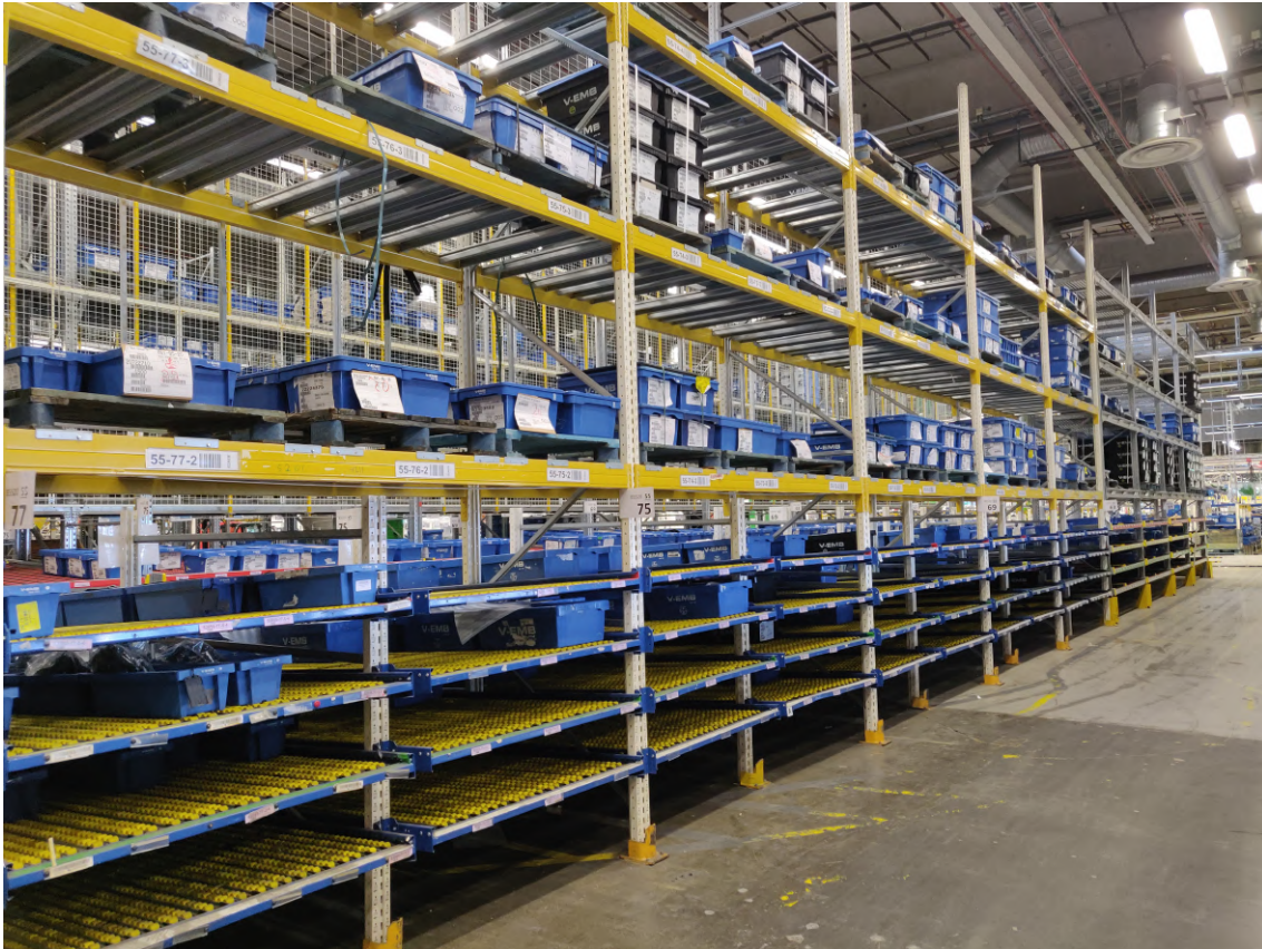
Figure 2.3: A pallet rack in the SuMa warehouse, the bottom level consist of four gravity-fed conveyors, while the upper three levels stores pallets with blue boxes.
