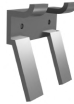
(b) Concept M2 , the upper hooks of the tool latch onto the front flange of the box, while the lower legs provide support on the bottom part of the box.
