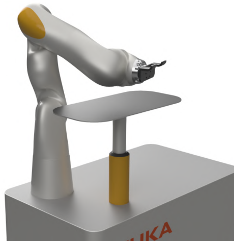
Figure 8.6: The drag tool working together with a lifting table, this solution adds extra complexity, but can handle heavier objects.
