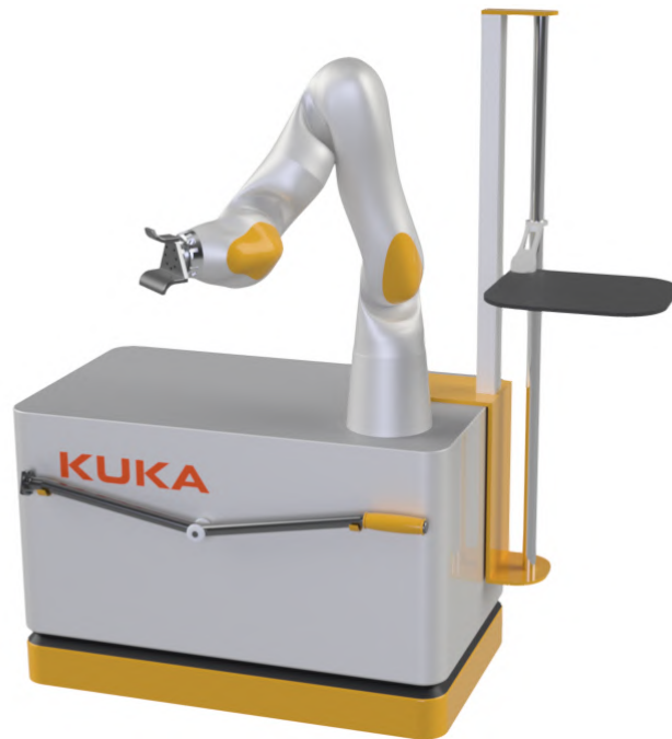
Figure 8.11: A complete solution able to alternate between two dimensions of its end effector by rotating it 180 degrees, as well as using a lifting table to support the weight of the boxes.
