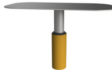
(d) Concept M3.2 , a table which can support the weight of a box while another tool drags it to the table, its adjustable along its vertical axis.
