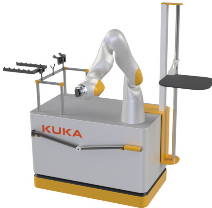
Figure 8.10: A complete solution able to switch between different tools, as well as using a lifting table to support the weight of the boxes.
