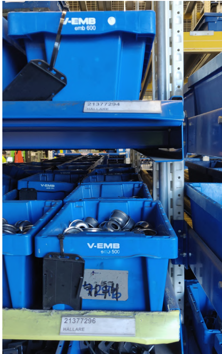
Figure 2.9: An image of two of the four layers of gravity-fed conveyors with boxes and the stop edges.
