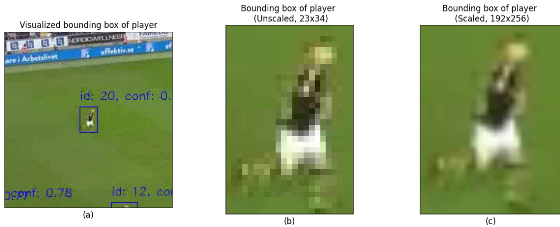
Figure 3.4: (a) the visualized bounding box of a selected player; (b) the extracted image patch of the player using the bounding box annotation; (c) the resized image patch after linear interpolation.
