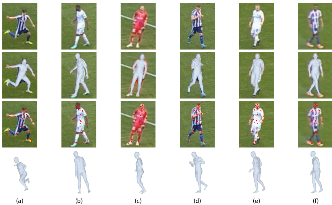
Figure 4.6: A selection of different poses and their subsequent pose estimates. Each column is a pose estimate case. The first row shows the original input bounding box after resizing. The second row shows the SMPL pose estimated by HMR2.0 projected onto the bounding box. The third row shows the projected SMPL joints. The final row shows a side view of the SMPL pose.
