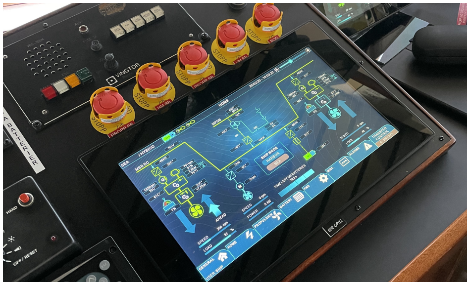
Figure 5.2: The battery indicator and emergency break buttons on Älvsnabben 4.
