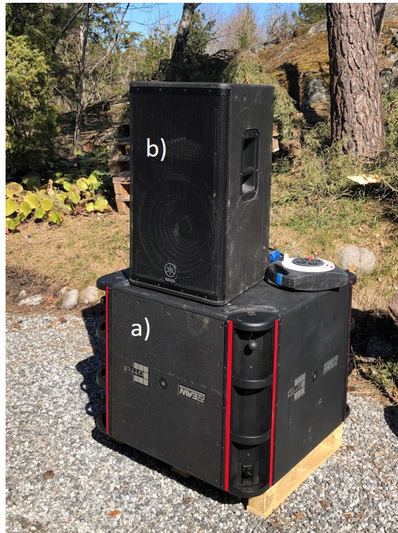
Figure 3.1: Speaker setup used during measurements, a) subwoofer EAW Otto™, b) loudspeaker Yamaha DHR 15.
