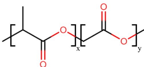
Figure 2.5 Molecular structure of poly(lactic-co-glycolic acid).
