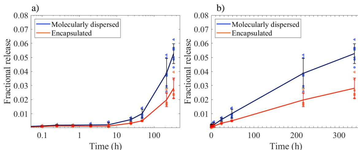
Figure 4.17 Release from coatings presented on a) a logarithmic time scale and b) a linear scale. The release from coatings with molecularly free biocide is compared to the release from coating with encapsulated biocide. Different marker symbols (triangles, circles and squares) indicate different release bath, 3 replicate release bath was studied for each coating formulation. The standard deviation of the released amount is indicated with error bars.
