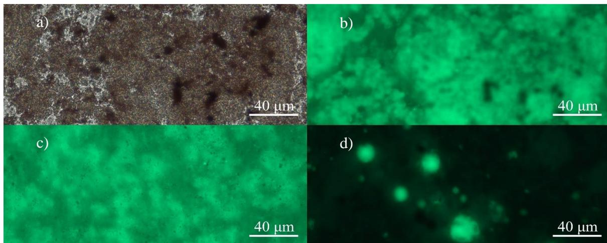
Figure 4.16 Microscopy images of the marine coatings. The top row shows unmodified, biocide-free, paint from Steen-Hansen in a) a brightfield micrograph, and b) a fluorescence micrograph. The bottom row displays fluorescence micrographs of reformulated Steen-Hansen paint, either containing c) molecularly free biocide, or d) encapsulated biocide.
