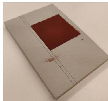
Figure 3.1 A polypropylene substrate coated at a 5 x 5 cm area.
