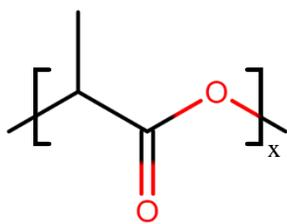
Figure 2.4 Molecular structure of polylactic acid.
