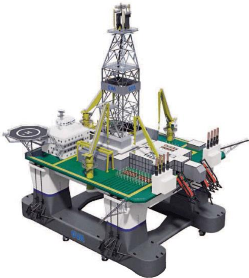
Figure 1.2 Semi-submersible drilling platform, courtesy of GVA Consultants.
