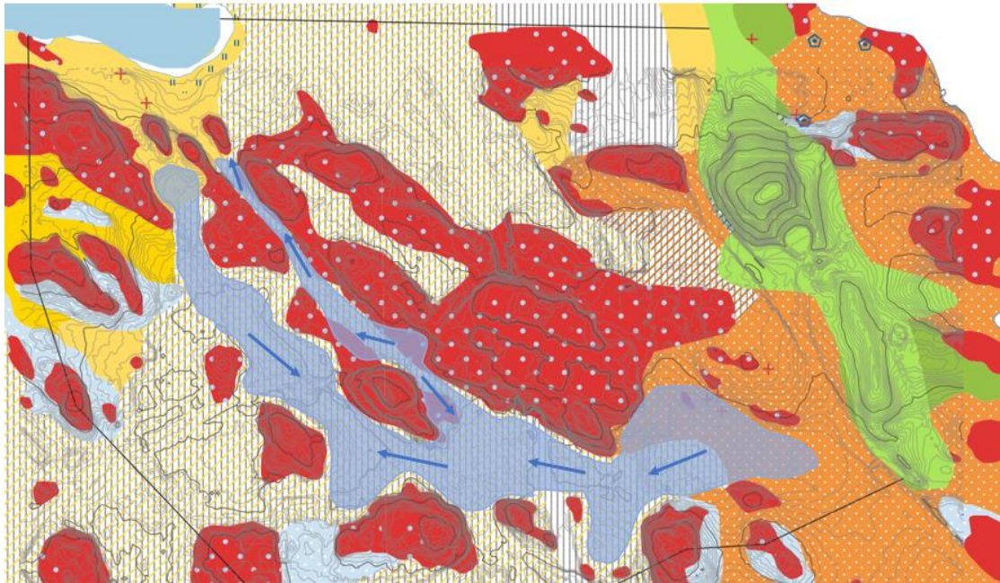
Figure B1. The estimated flow direction of the confined aquifer based on previous hydrogeological investigations performed in the area.
