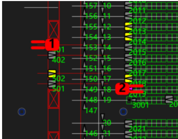
Figure 4.4: Lock-zone method's deadlock situation: two AGVs go out of stations at the same time and the next nodes are close to each other.
