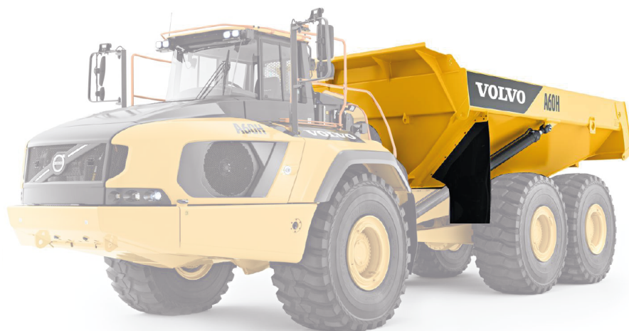
Figure 1.1: Articulated hauler with the hauler body highlighted (Volvo AB, 2022).
