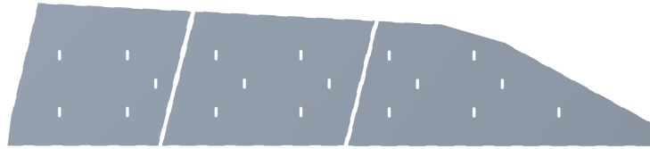
Figure 5.33: Example of how the wear plates can be divided into several plates to reduce the separate plate weight and enable a higher degree of automation.
