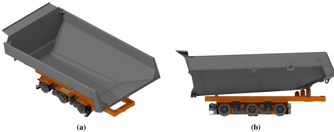
Figure 5.38: A hauler body loaded onto the fixture and AGV.
