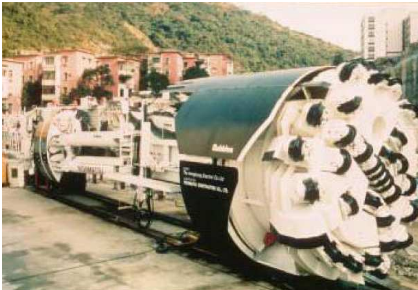
Figure 1 A tunnel boring machine with disc cutters. Gertsch et al (2002)
