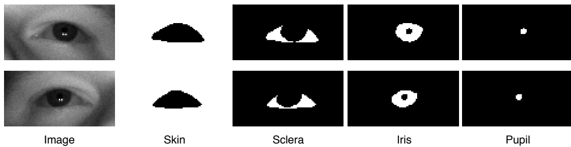
Figure 3.12: Image portraying the masks extracted from the eye-image. A white colour (binary one) in the masks corresponds to the specific class (named at the bottom of image) while black (binary zero) corresponds to 'something else'. Glint(s) and glare(s) are not included in these images.
