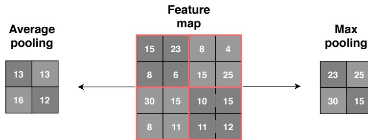
Figure 2.2: The resulting maps after max and average pooling on a feature map.
