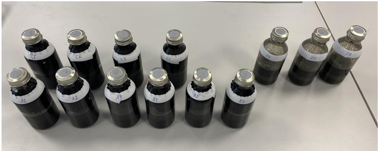
Figure 3.6 Sealed test reactors after the addition of inoculum, substrate and additives at the start of first phase of the experiment.
