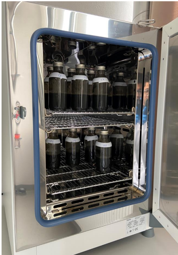
Figure 3.7 Maintenance of test reactors inside an incubator at 55 °C.
