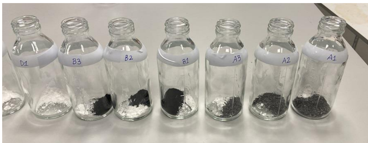
Figure 3.5 Test reactors after receiving 1.5 g substrate and 7.5 g additive at the start of first phase of the experiment.
