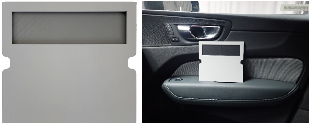
Figure 11, A plaque holder. On the right with two Charcoal Solid plaques inserted.
