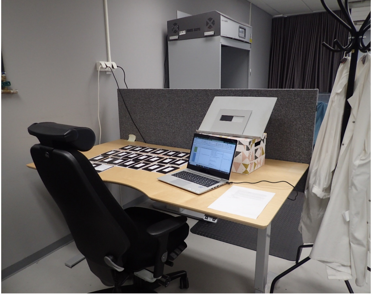
Figure 21, Test setup with screen to hide view of plaques from participants. The light booth can be seen in the background.
