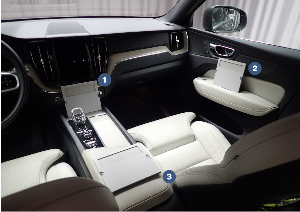
Figure 12, The 3 final plaque holders placed on their correct positions in the car. Described more in detail in the text above.
