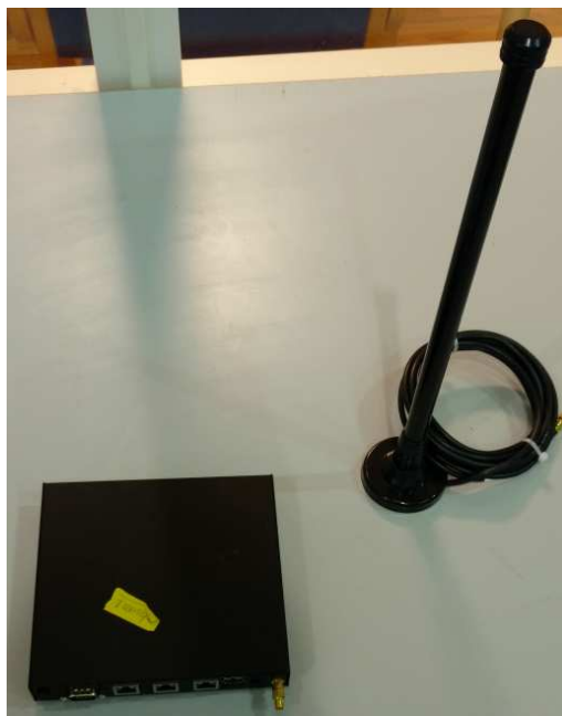
Figure 3.2: The Figure is taken of the hardware setup of the communication system. The computer is of model PC engines APU with wireless network card based on Atheros AR92xx. The antenna is from MobileMark of model ECOM9-5500 which operates on frequencies of 5-6 GHz and was measured to have a secure range up to 200 m.
