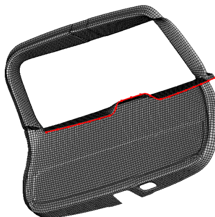
Figure B.5: Boundary line on tailgate panel used for analysis of results obtained from sun simulation.
